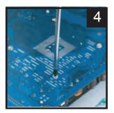
Insert the screws from the back of the motherboard and tighten them.
