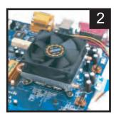
Place the cooler and align it with the holes of the motherboard.
