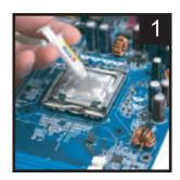
Apply the thermal grease evenly to the CPU.
