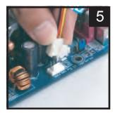
Connect the fan's connector to the motherboard.
