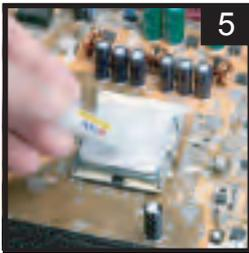
Place the washers over the AM2 screws and use the screws to tighten the mounting parts from the back of the motherboard
