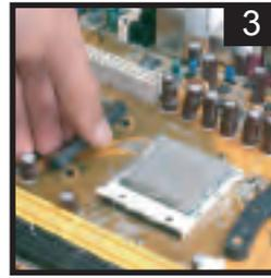
Place the mounting parts and aim at the mounting holes.
