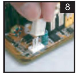
Connect the fan's connector to the motherboard.
