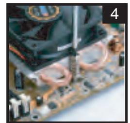
Tighten the cooler with the K8 spring screws.
