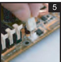
Connect the fan's connector to the motherboard.
