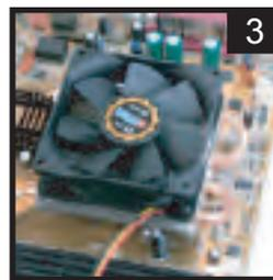
Place the cooler and align it with the holes.
