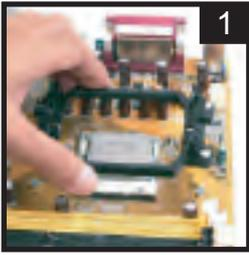
Remove the screws and the retention frame.
