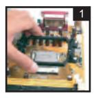
Remove the screws and the retention frame.
