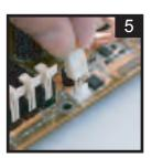
Connect the fan's connector to the motherboard.
