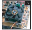
Place the cooler and align it with the holes.
