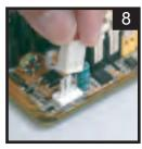
Connect the fan's connector to the motherboard.
