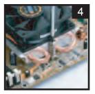
Tighten the cooler with the K8 spring screws.
