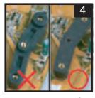
The concavity faces downward. (Correct) The concavity faces upward. (Wrong)
