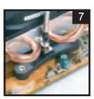
Place the cooler and align it with the holes.
